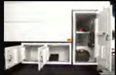
Small, lockable storage compartments (left) and a large pass-through compartment (right) accommodate a variety of equipment.
