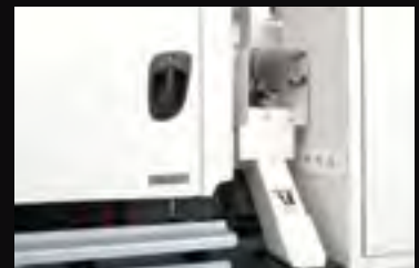
Clear back of cab allows the installation of outriggers, mid-ship aerials and other body components.
